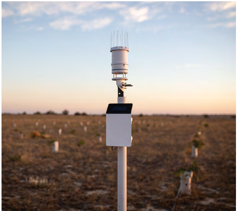
This weather station at Jarrega, supported by Edaphic Scientific, provides crucial data to Greening Australia's seed science team about optimising native seed production area establishment.
