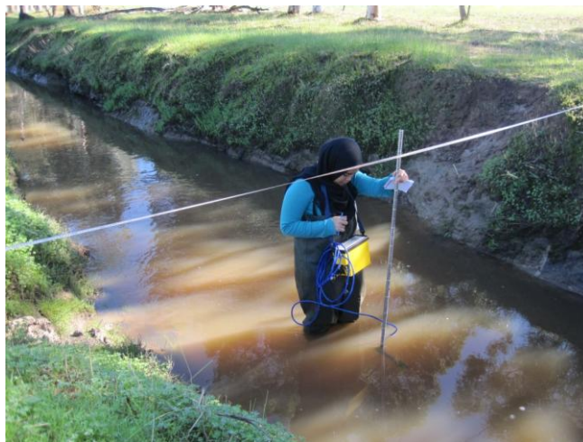
UWA Honours student Miss Hani Mohamad conducted flow velocity measurements in the drain at Site 1 to measure the exchange of water between the groundwater table and the drain.
