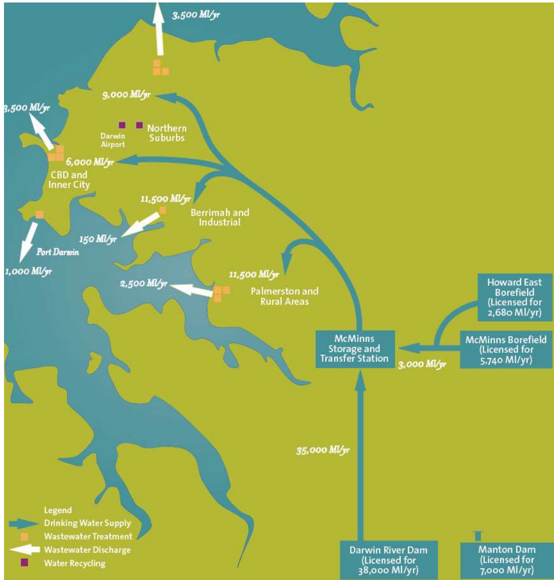
Figure 34 Darwin's water and sewerage infrastructure showing the relative amounts of water pumped from Darwin River Dam and McMinns/Howard East Borefields to supply Darwin with water. Quantities shown are from 2006. Source: Power and Water Corporation (2006a)
