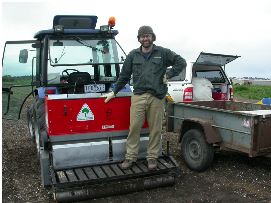
Figure 7. The seeding machine used to restore GGRP sites was an adapted AERA-vator ® (1st Products Inc., Tifton, GA, USA). The seeder operator in this image is Rod White, then manager of the Moolapio programme. (Photo Paul Gibson-Roy).
