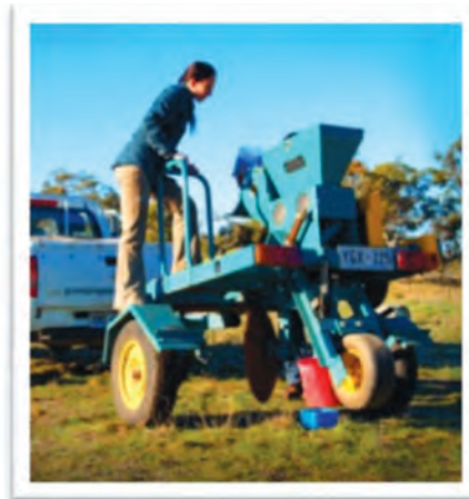
Photo 6. A direct seeder with a large disc that scalps a clean seed bed. Note the single calibrated seed box on top and press wheel at the bottom rear. This disc seeder is particularly suited to lighter soils and requires little horsepower (e.g. a ute).
