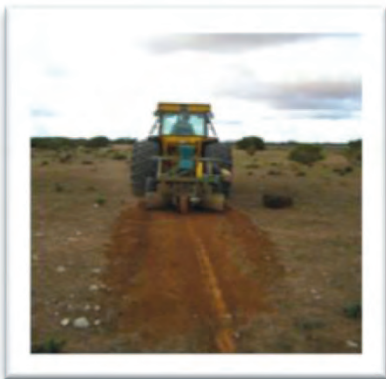
Photo 14. A V blade seeder mounted on a tractor creating a suitable seed bed for native species. This robust machine is particularly suited to stony sites such as this one.
