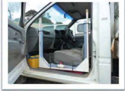
Photo 12. Planting or seeding trees and shrubs on the contour minimises erosion and helps retain rainfall. This 'level-ometer' filled with water is a simple and inexpensive way to accurately drive along on the contour with a spray rig or direct seeder (Photo 15).
