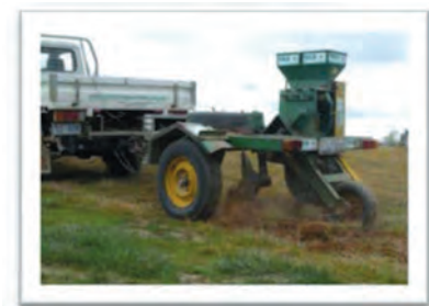
Photo 15. A traditional single row direct seeder in action. The large disk at the front scalps away a strip of topsoil to reduce weeds and remove excess nutrients. A mixture of seeds and a bulking agent (e.g. sand) are then gravity fed through a tube in front of the press wheel that ensures good seed to soil contact.
