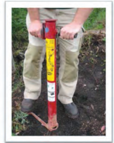
Photo 13. This tool (Pottiputki) can be used to hand plant many hundreds of seedlings a day. Pushing down on the tool creates a slot in the soil, then the seedling is dropped down the tube. This tool saves having to bend down to plant.
