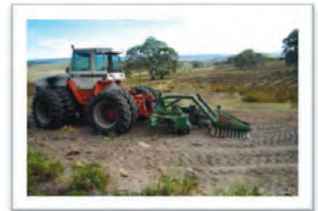
Photo 10. This heavy duty machinery has been developed by the commercial plantation industry to improve tree seedling establishment in soils prone to water logging.
