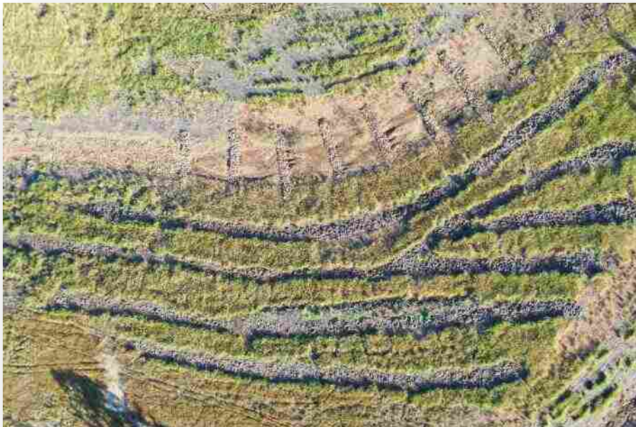
Plate 23 Hay and debris bunds inter-sown with exotic grass seed on the downstream eastern batter of Treatment 8 proved very effective for stabilising long low slope batters.
