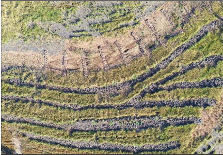
Plate 16 Debris and hay bunds installed on the contour in Treatment 8
