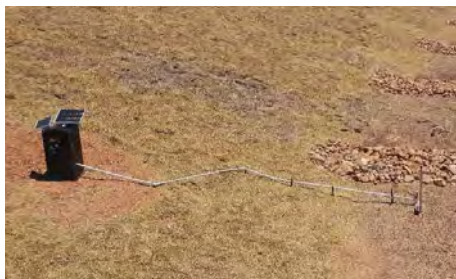
Treatment 3: Integrated water quality sample station on a treated gully. Photo credit: Fruition Environmental
