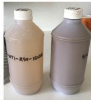
Water quality samples taken from the treated gully (left) and control/untreated gully (right).
