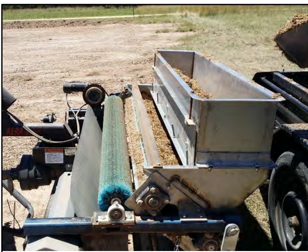
Image 1. Rebuilt seed hopper with belt that raises seed up and out of the hopper. This ensures there is no bridging or blocking of seed/chaff, while still allowing regulation of seed flow.
