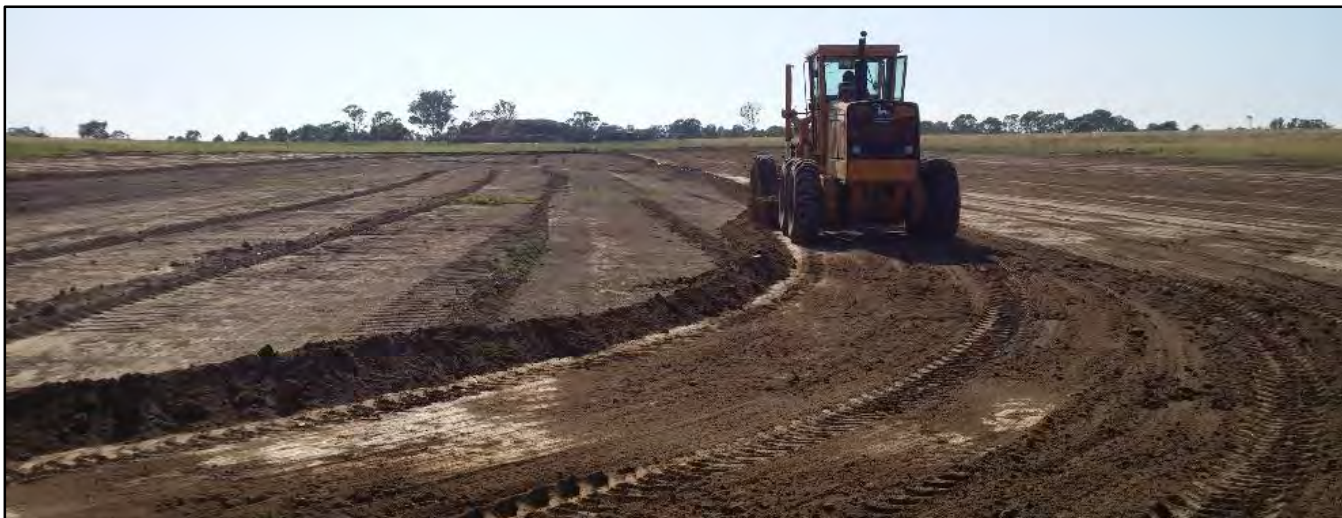
Image 6. Tony comes in with a road grader after Wayne has finished scalping to 'clean up' the surface in readiness for seeding.
