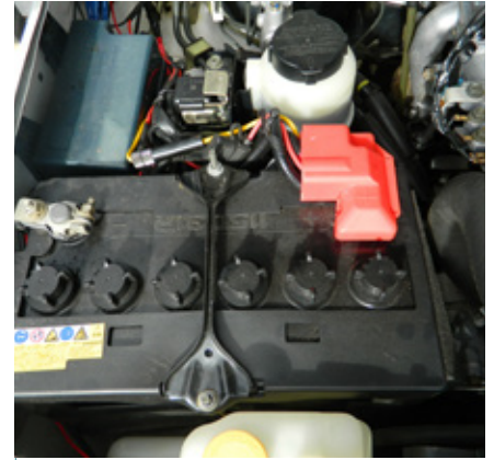
This battery is not sealed. You can remove the caps.
